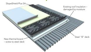
**Re-Roofing:** Installing SlopeShield Plus SA on new thermal board applied over existing insulation allows for the drying and reuse of existing insulation.
