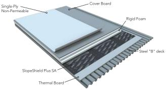
**Typical Roof Cross-Section:** Apply SlopeShield Plus SA to top of thermal board.
