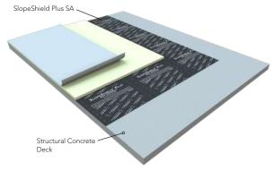
**Structural Concrete Deck:** SlopeShield Plus SA can be applied over green concrete or a damp existing concrete and lightweight insulating concrete roof decks, provided the surface complies with a bull float finish or better.
